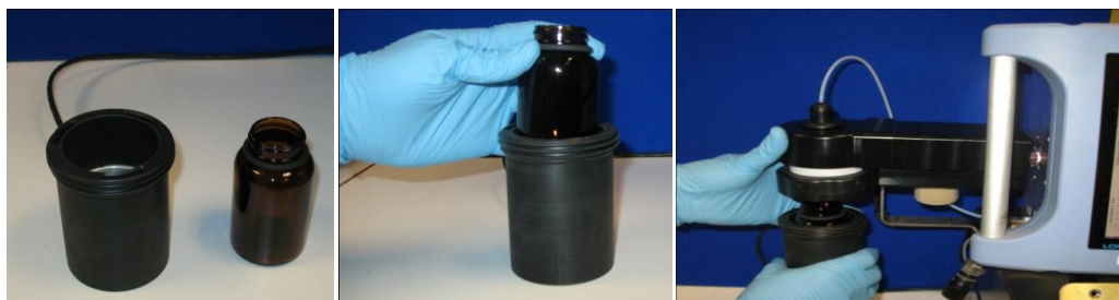
Figure 2 – Loading sample bottle
